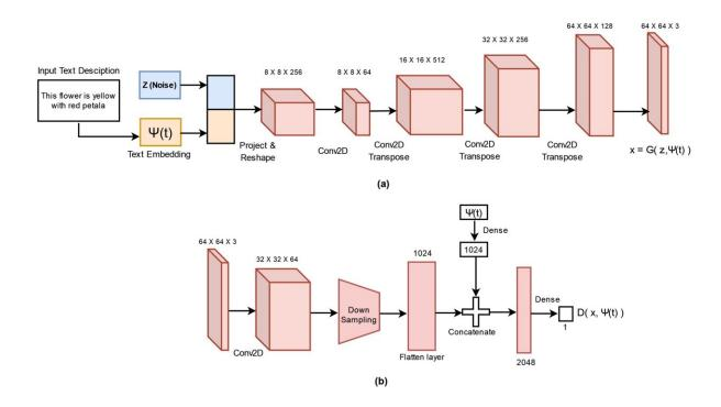
The proposed T2CI-GAN Model-1 architecture using backbone networks. (a) Generator network and (b) Discriminator network. Credit: https://arxiv.org/abs/2210.03734
