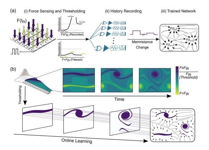
a) i) Neuromorphic metamaterial composed of mechanosensing unit cells with inherent filtering, transduction, mechanoelectric signal amplification, and
