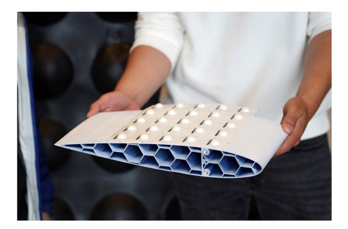
Arrays of domes on a drone wing may help it to detect information from its surroundings only when necessary. Credit: Purdue University/Jared Pike
