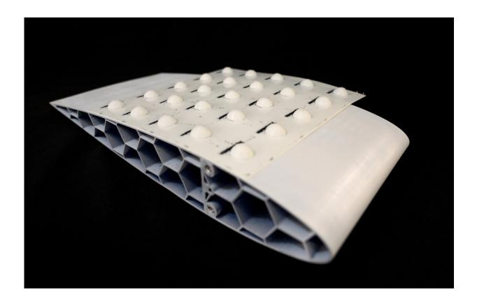
Researchers have discovered a new possible use for the dome shape that you would find on a to-go cup lid. Patterns of these invertible domes on a drone's wings would give it a way to remember in microseconds what dangerous conditions feel like and react quickly. Credit: Purdue University/Jared Pike
