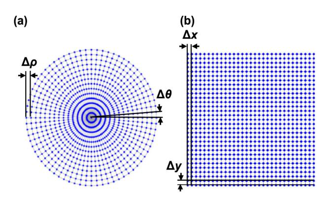
Layouts of control point clouds generated by (a) ring method (b) mesh method. Credit: *International Journal of Extreme Manufacturing* (2022). DOI: 10.1088/2631-7990/ac5f12
