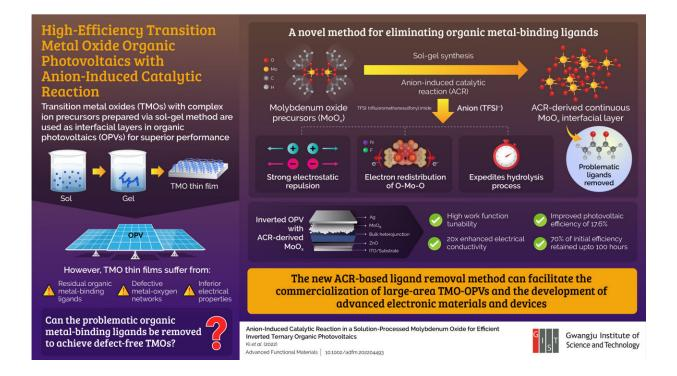
Researchers from GIST report ACR as an effective way of removing unwanted ligands and improving the efficiency of organic photovoltaics (OPVs) with a transition metal oxide (TMO) interfacial layer. Credit: Kwanghee Lee from Gwangju Institute of Science and Technology, Korea
