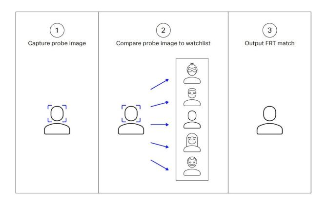
The process of using facial recognition for identification, or one-to-many facial recognition. First, a probe image of a person is captured. Then, the probe image is compared with a watchlist of known facial images to determine if there is a match. Credit: *A Sociotechnical Audit: Assessing Police Use Of Facial Recognition*, Evani Radiya-Dixit, October 2022
