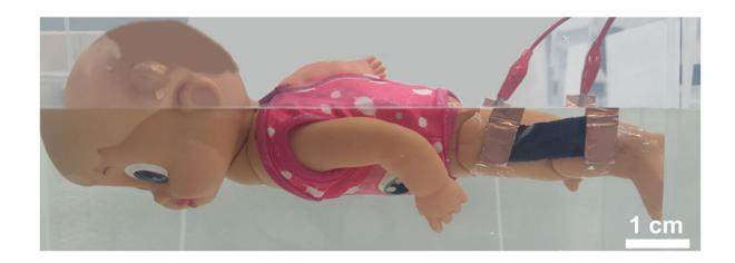
An underwater movement sensor attached to a motorized swimming doll's knee alerts a smartphone app when the doll stops kicking, simulating a swimmer in distress. Credit: *ACS Nano* (2022). DOI: 10.1021/acsnano.2c08325
