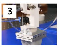
(Upper) Gripping objects of various sizes(Lower) The gripper is used to grip an acupuncture needle placed on the floor. In the gripping process, the tip of the gripper bends like a finger, comes in contact with the floor, and then picks up the acupuncture needle. Credit: Korea Institute of Machinery and Materials (KIMM)
