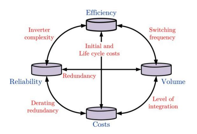
Trade-off between the power electronic performance parameters. Credit: *IEEE Open Journal of Power Electronics* (2022). DOI: 10.1109/OJPEL.2022.3204630
