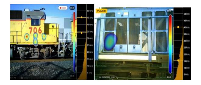
SwRI developed an automated compressed air leak detection system that can acoustically and visually detect and report air leaks on moving trains, indicated by spectral signatures in the photos. The team tested the proof-of-concept system on rail cars and trains at SwRI's Locomotive Technology Center in San Antonio. Credit: Southwest Research Institute
