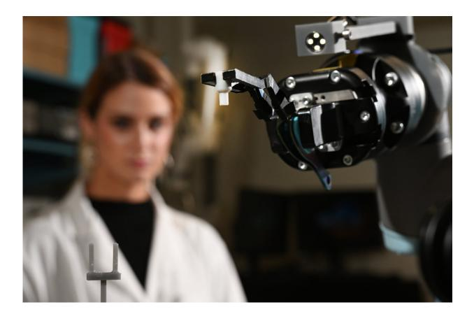
The robotic arm automatically positions samples within a hot cell according to both the sample attributes and the type of examination being performed. Credit: Idaho National Laboratory
