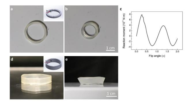
(a, b) The ring with equal thickness (t) and height (h) can only snap twice and shrink to the minimum size. (c) The simulated flipping reaction moments of a ring with radius 15 mm through FEA. (d, e) The ring with h = 5t (d) transforms into a static trumpet-like shape when placed on hot surface without snapping (e). Credit: *Advanced Materials* (2022). DOI: 10.1002/adma.202207372
