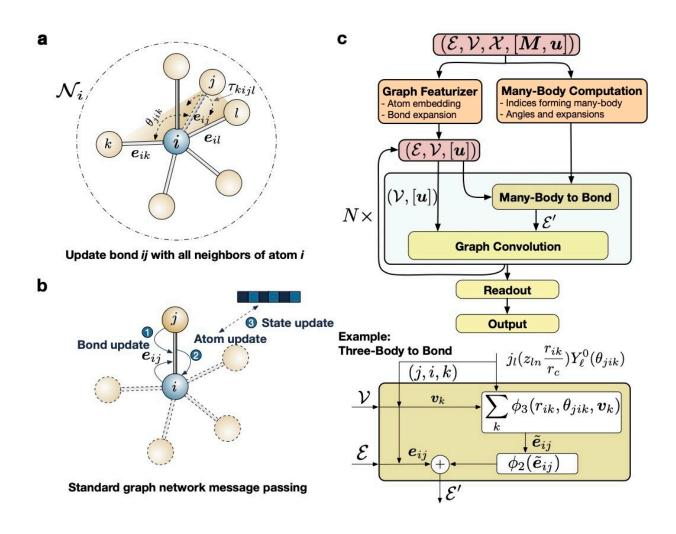
The model architecture starts from a position-included graph, and then goes through a featurization process, followed by main blocks, and the readout module with energy, force and stress outputs. The featurization process consists
