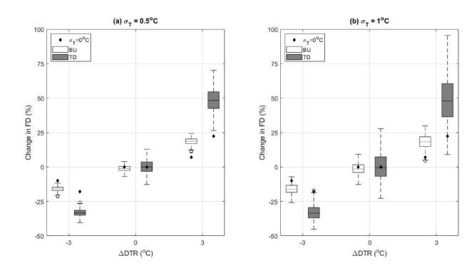
Distribution of change in fatigue damage as compared to the existing climate for different climate change scenarios assuming a standard deviation of (a) 0.5°C and (b) 1°C for the 250 mm thick pavement in Phoenix, AZ. Credit: *Results in Engineering* (2022). DOI: 10.1016/j.rineng.2022.100736
