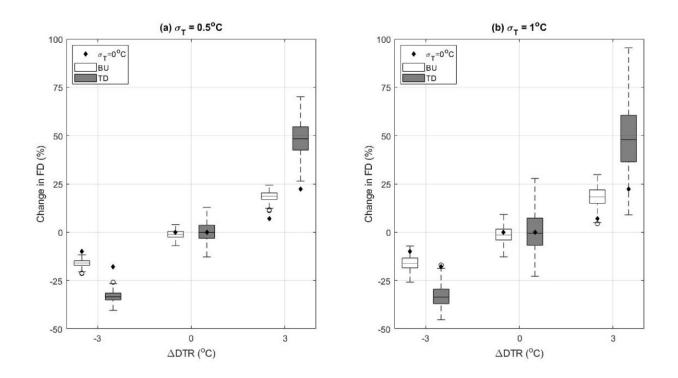
Distribution of change in fatigue damage as compared to the existing climate for different climate change scenarios assuming a standard deviation of (a)  $0.5^{\circ}$ C and (b) 1°C for the 250 mm thick pavement in Phoenix, AZ. Credit: *Results in Engineering* (2022). DOI: 10.1016/j.rineng.2022.100736
