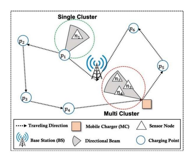
In a new study, researchers from Chung-Ang University proposed a new energyefficient adaptive directional charging (EEADC) algorithm that considers the
