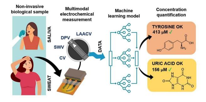
Combining machine learning with multimodal electrochemical sensing can improve the analytical performance of biosensors and benefit non-invasive health monitoring, such as testing that involves sweat or saliva. Credit: Provided by Vinay Kammarchedu
