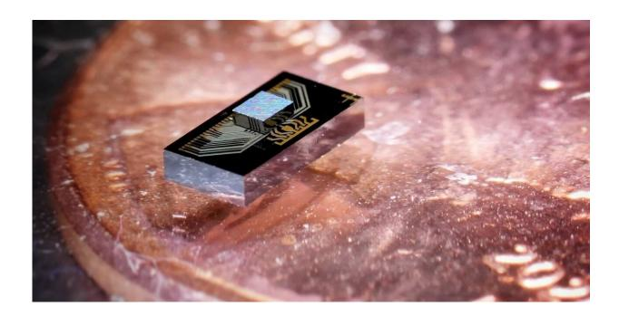
The chip sandwich: an electronics chip (the smaller chip on the top) integrated with a photonics chip, sitting atop a penny for scale. Credit: Arian Hashemi Talkhooncheh
