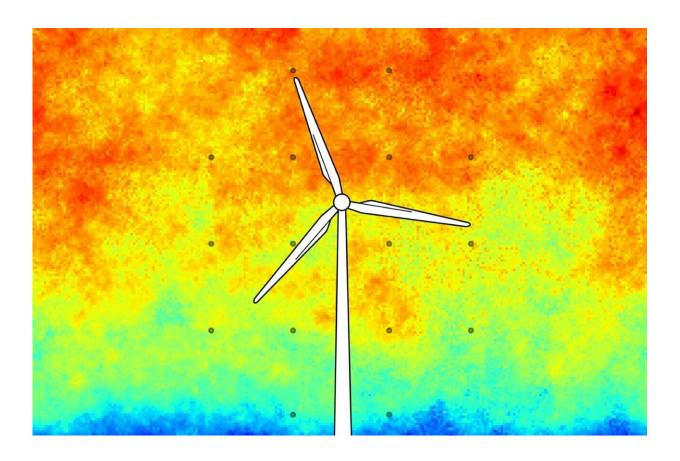
Using the data from 16 anemometers (indicated as grey dots) that were in operation at two measuring stations near the German North Sea coast in the 1980s, the team reconstructed a complete, three-dimensional wind field with the help of the new model. Here, a section can be seen. Blue and green hues represent low wind speeds, yellow and red hues represent higher wind speeds. Credit: University of Oldenburg/Jan Friedrich
