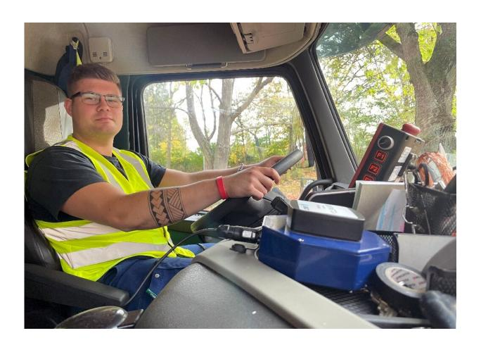
The trucks have been fitted with a device that measures the signal quality on their routes.
