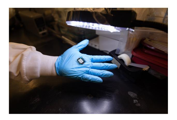
This prototype all-perovskite tandem solar cell measures one square centimeter and has a power conversion efficiency of 27.4%, which is higher than is currently possible with traditional single-junction silicon solar cells. Credit: Aaron Demeter / University of Toronto Engineering
