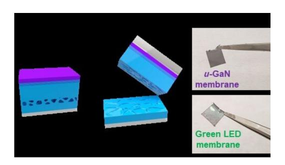
Representative schematic illustration and digital camera images for microcavityassisted crack propagation and its corresponding undoped-GaN and green LED membranes, respectively. Credit: Compuscript Ltd
