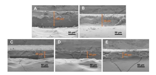
The cross-section SEM images of the shape memory films with different spinning coating rotational speed (A) 2000 rpm, (B) 3000 rpm, (C) 4000 rpm, (D) 5000 rpm and (E) 6000 rpm. Credit: *Nano Letters* (2022). DOI: 10.1021/acs.nanolett.2c03645
