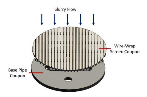
Southwest Research Institute has created and validated new microscopy methods to evaluate erosion in sand screens used in oil and gas production wells. The methods studied the effects of sand-laden slurries as they passed through wire-wrapped sand screens, particularly how the screen erodes as particles pass through the screen gaps. Credit: Southwest Research Institute
