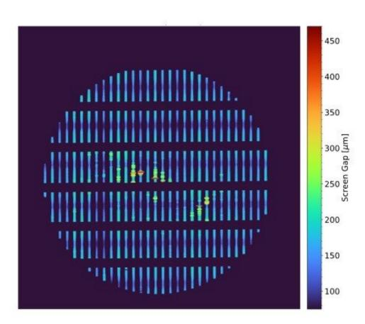
Southwest Research Institute used image microscopy to create a more effective, comprehensive method of characterizing erosion in wire-wrapped sand screens
