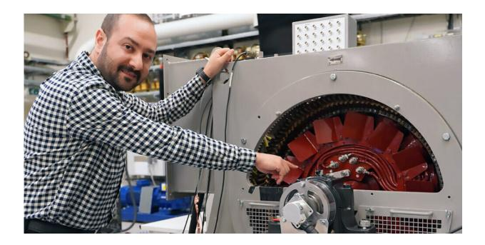
Hossein Ehya has used a specially built model of a generator to carry out experiments in NTNU's SmartGrid laboratory. Credit: Juliet Landrø/HydroCen
