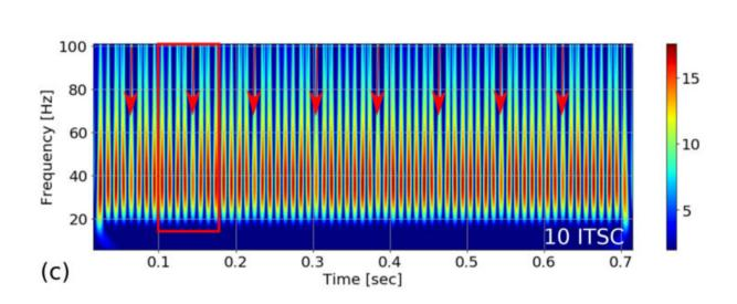
Here the signals show that one of the coils has a short circuit. Both the strength and length of the bar showing the broken coil are reduced. Credit: Norwegian University of Science and Technology
