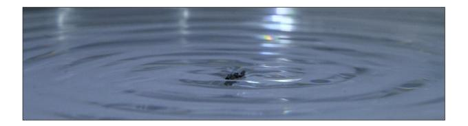
Vortex generation by multiple swimming robots. The diameter of the multiple robots is 460 µm. Credit: S. Won, et al., *Nature Communications*, 13, 6750 (2022)
