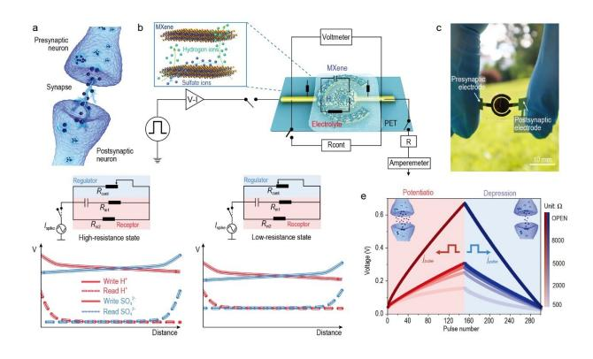
(a) Structural and functional illustration of the biological synapse. (b) Illustration of the FMES device. Inset shows dynamic diffusion process. (c) Optical image of the FMES device. (d) Schematic explaining the corresponding circuit diagram and the decoupling of the read and write operations. (e) Monitored postsynaptic current under several sequential voltage pulses. Credit: *Science China Press*
