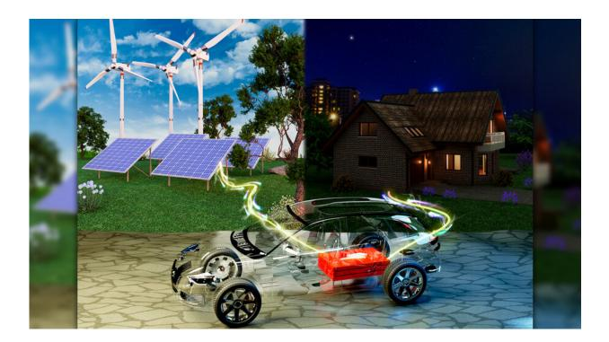
In the future, electric vehicles could boost renewable energy growth by serving as "energy storage on wheels"—charging their batteries from the power grid as they do now, as well as reversing the flow to send power back and provide support services to the grid. Credit: Ehsan Faridi and Ehsan Keshavarzi/Inmywork Studio
