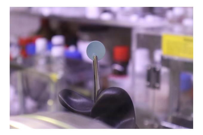
A 0.1 mm thick PMC solid electrolyte composed of a polymer matrix, ceramic and MOF. It is designed to improve fire safety compared to commercial liquid electrolytes. Credit: Andrew Johnston, IMDEA Materials Institute.
