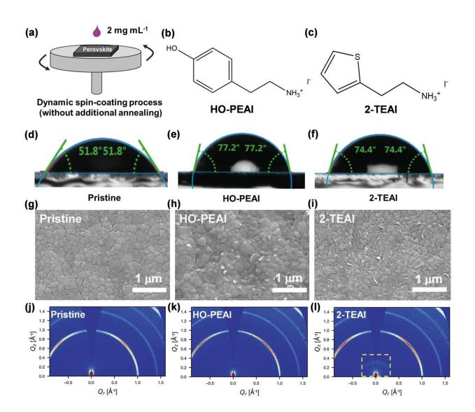
Properties of perovskite films without and with surface modulators. a)
