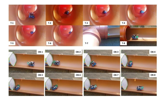
Joey moving through the experimental pipe network. T-1 through T-8: moving through T-junction. OB-1 through OB-8: reaching an obstruction and turning back. Credit: TL Nguyen, A Blight, A Pickering, A Barber, GH Jackson-Mills, JH Boyle, R Richardson, M Dogar, N Cohen
