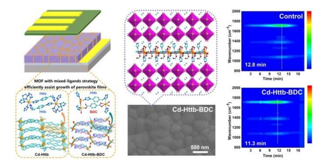
A novel MOF (Cd-Httb-BDC) designed via a mixed-ligands strategy was used as a heterogeneous nucleation center to simultaneously passivate deep-level defects and assist the crystallization of high-quality perovskite films with enlarged grain size towards the development of efficient and stable PSCs. Credit: *Journal of Energy Chemistry*
