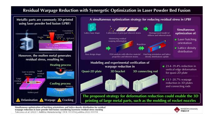
Researchers from Japan and the USA propose a deformation reduction strategy in LPBF-based additive manufacturing involving a synergetic optimization of laser hatching orientation and lattice density distribution. Credit: Akihiro Takezawa from Waseda University, Japan
