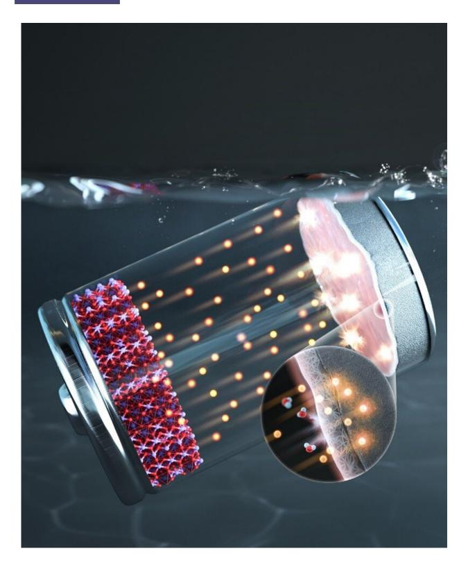
Schematic diagram of an aqueous zinc battery stabilized by a protective polymer layer. Credit: POSTECH
