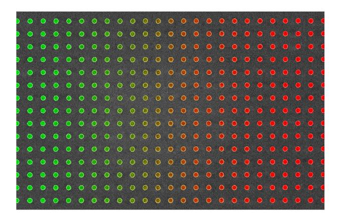
The new sensor is based on an optical phenomenon, plasmons, which occur when metal nanoparticles capture light and give the particles a distinct color. This color changes when the amount of hydrogen in the surroundings varies and the sensor can alarm at critical levels. Credit: Chalmers University of Technology | Yen Strandqvist
