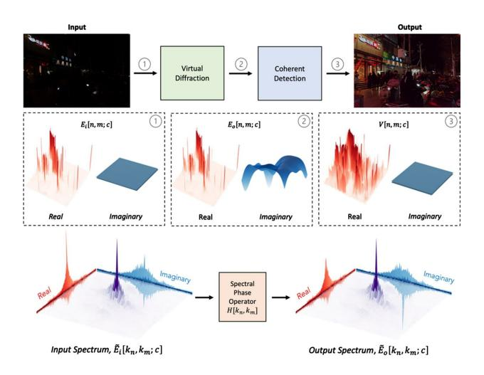
Physical interpretation of the VEViD algorithm showing its impact in spatial domain (top row) and in spectral domain (bottom row). In spatial domain, the real part of the image is nearly unchanged whereas an imaginary part is created after diffraction. This observation supports the mathematical approximation in the latter part of the paper. Credit: *eLight* (2022). DOI: 10.1186/s43593-022-00034-y
