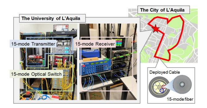
15-mode multiplexed network constructed on the testbed in the city of L'Aquila, Italy. Credit: National Institute of Information and Communications Technology (NICT)
