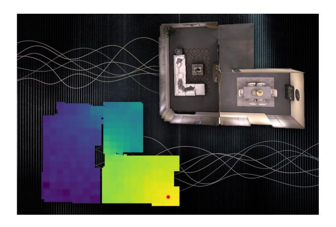
MIT researchers have developed a machine-learning technique that accurately captures and models the underlying acoustics of a scene from only a limited number of sound recordings. In this image, a sound emitter is marked by a red dot. The colors show the sound volume if a listener were to stand at different locations — yellow is louder and blue is quieter. Credit: Massachusetts Institute of Technology
