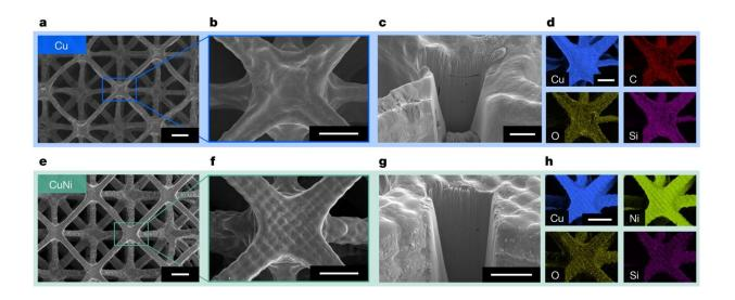
Morphology of Cu and CuNi microlattices. a–c,e–g, SEM images of Cu (a–c) and CuNi (e–g) octet lattices, showing multiple unit cells from the top (a,e), a single node (b,f) and a FIB-milled cross-section showing the internal structure of a node from 52° tilt (c,g). d,h, EDS elemental mapping, showing uniform distribution of Cu (d) and uniform distribution of Cu and Ni (h). Scale bars: a,e, 100 μm; b,f, 50 μm; c,g, 20 μm; d,h, 50 μm. Credit: *Nature* (2022). DOI: 10.1038/s41586-022-05433-2
