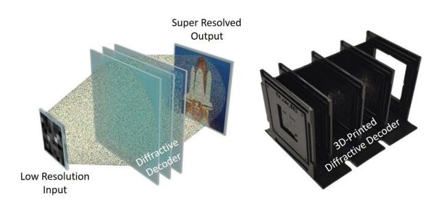
Super-resolution image display using diffractive decoders. Credit: Ozcan Lab @ UCLA.
