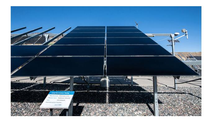
A 0.6KW First Solar Cadmium Telluride PV test array, installed June 1995 at NREL's Outdoor Test Facility. Credit: Dennis Schroeder, NREL
