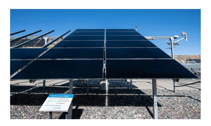
A 0.6KW First Solar Cadmium Telluride PV test array, installed June 1995 at NREL's Outdoor Test Facility. Credit: Dennis Schroeder, NREL
