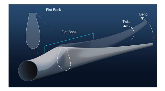
A digital rendering shows a modern bend-twist, flat-backed wind turbine blade. A cross-sectional view of the flat back is shown in the upper left corner. Credit: Besiki Kazaishvili, NREL
