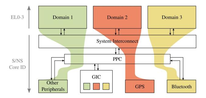
High-level overview of domain isolation in TEEtime: Access to peripherals is enforced with a partition controller (PPC). The interrupt controller (GIC) is shared among domains, such that all domains can handle interrupts concerning their peripherals. Credit: Groschupp et al.
