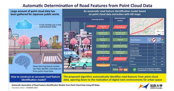
Researchers from Japan propose, in a new study, a deep learning-based algorithm that can automatically extract road features from point cloud data using high-precision 3D maps. The proposed model could help with maintenance of roads and the preparation of faithful road maps in virtual space or a digital twin environment. Credit: Ryuichi Imai from Hosei University, Japan
