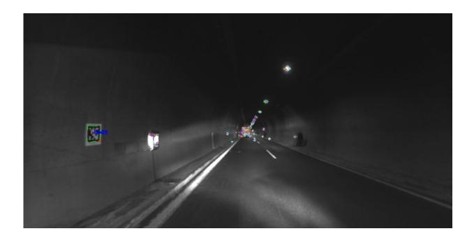
This photo was taken using a camera mounted on a robot vehicle. The robot navigates through the tunnel using a series of markers (shown in colour in the photo). The markers are then processed by a positioning algorithm. Credit: SINTEF
