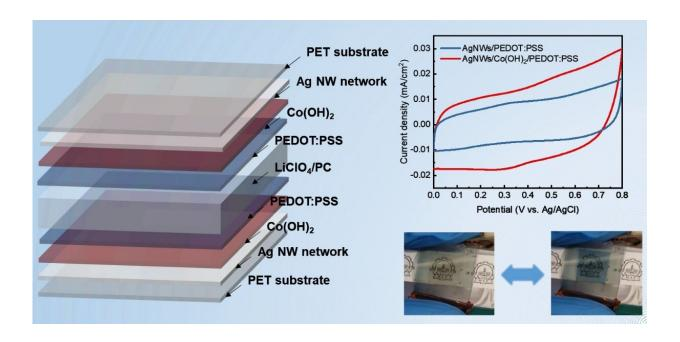
An electrochromic supercapacitor was realized using silver nanowire electrodes as the current collector. PEDOT:PSS was used not only as the functional layer to achieve electrochromic and energy-storage properties at the same time, but also as a protective layer to prevent silver nanowires from electrochemical corrosion. Credit: *International Journal of Extreme Manufacturing* (2022). DOI: 10.1088/2631-7990/aca638
