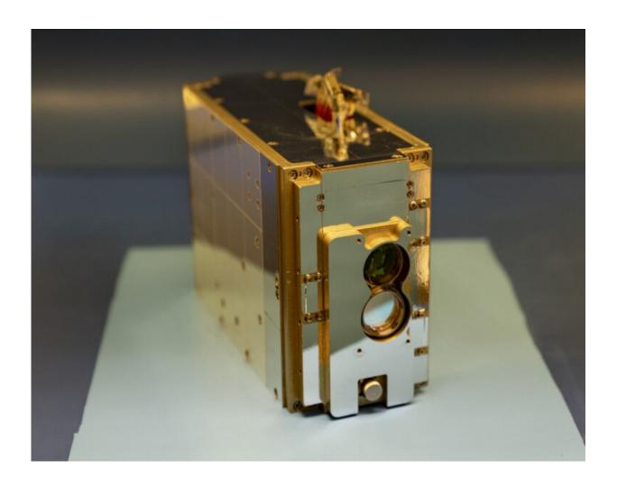
The TBIRD communications payload, pictured above, is showcasing unprecedented data rates for space-to-ground laser communications. Credit: Lincoln Laboratory
