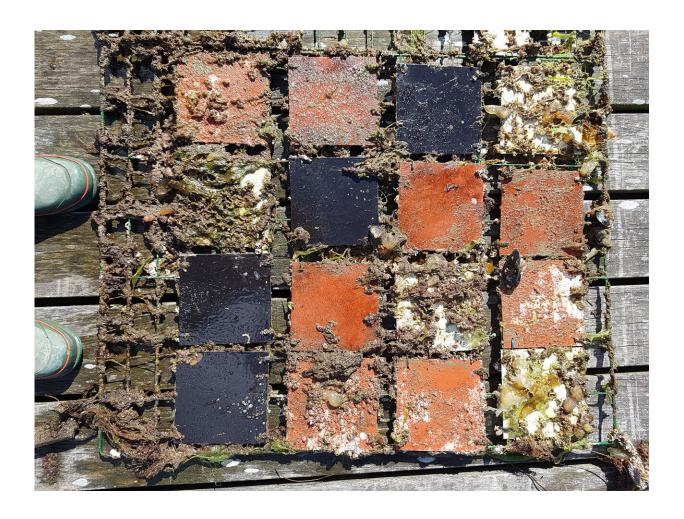
A Chalmers-led study shows that an environmentally friendly antifouling paint is more effective against fouling than a traditional copper-based paint. The black surfaces are coated with biocide-free silicone-based paint, the red surfaces are coated with copper-based paint and the white surfaces have no antifouling treatment. The picture was taken after two years of exposure in the sea. Credit: IVL | Anna-Lisa Wrange
