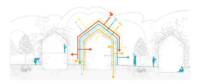
The ecolope, designed by transforming a conventional building envelope into a dynamic living space for animals, plants and even microbiota. It modulates environmental conditions such as sunlight and water/humidity, thereby creating and connecting habitats and improving human well-being (unscaled diagram). Credit: *People and Nature* (2022). DOI: 10.1002/pan3.10411
