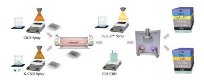
Incheon National University researchers report an eco-friendly, cost-effective, scalable fabrication technique for high-efficiency copper indium gallium sulfur diselenide solar cells, which uses aqueous spray deposition in air environment and avoids expensive vacuum conditions. Credit: JunHo Kim, Incheon National University
