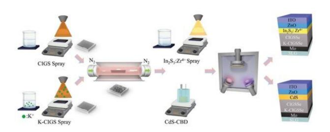
Incheon National University researchers report an eco-friendly, cost-effective, scalable fabrication technique for high-efficiency copper indium gallium sulfur diselenide solar cells, which uses aqueous spray deposition in air environment and avoids expensive vacuum conditions. Credit: JunHo Kim, Incheon National University
