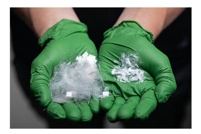
NREL/UoP's enzymatic recycling platform efficiently deconstructs raw PET plastic (left) into its chemical building blocks. The PET sample on the right has lost 97.7% of its mass after being broken down by NREL/UoP's enzymes. Credit: Dennis Schroeder, NREL
