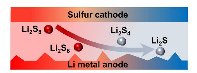
The violent exothermic reactions between high-order polysulfide rather than lower-order polysulfide and dendritic Li push the cycled Li–S pouch cells into thermal runaway. Credit: Fengni Jiang, Taiyuan University of Technology
