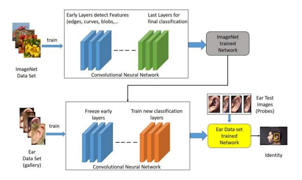
An overview of the deep learning-based ear recognition system. The proposed CNN is pre-trained on the ImageNet dataset and then fine-tuned using an ear dataset. Credit: *IEEE Access* (2022). DOI: 10.1109/ACCESS.2022.3206024
